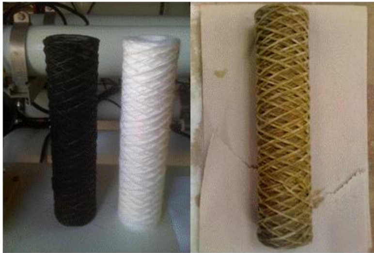
Figure 5-34: Cartridge Filter Taken out of NF Pilot (left), New Cartridge Filter (middle) and Cartridge Filter after Exposure to Atmosphere (right)
