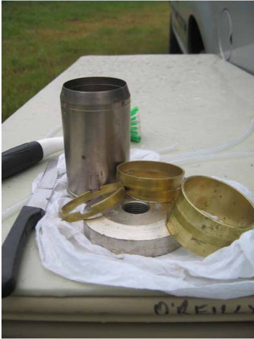
Figure 3: Outer and Inner Cylinders for the Hammer-Drive Core Sampler
