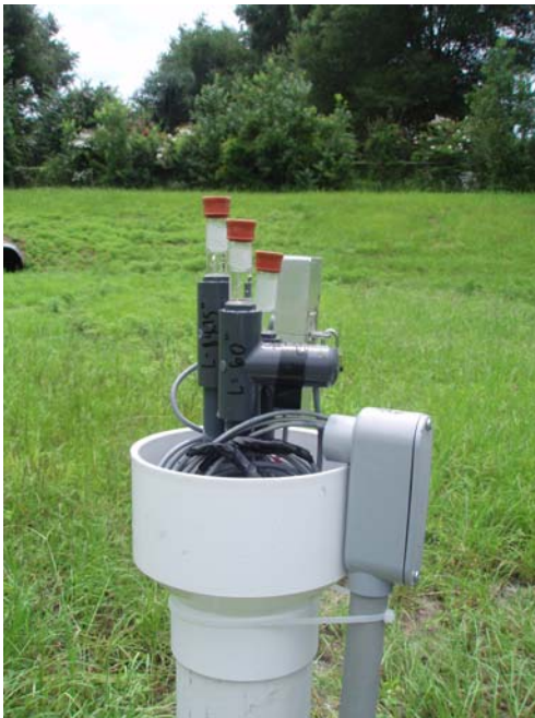
Figure 6: Above ground configuration of the tensiometer (pressure-sensing device)
