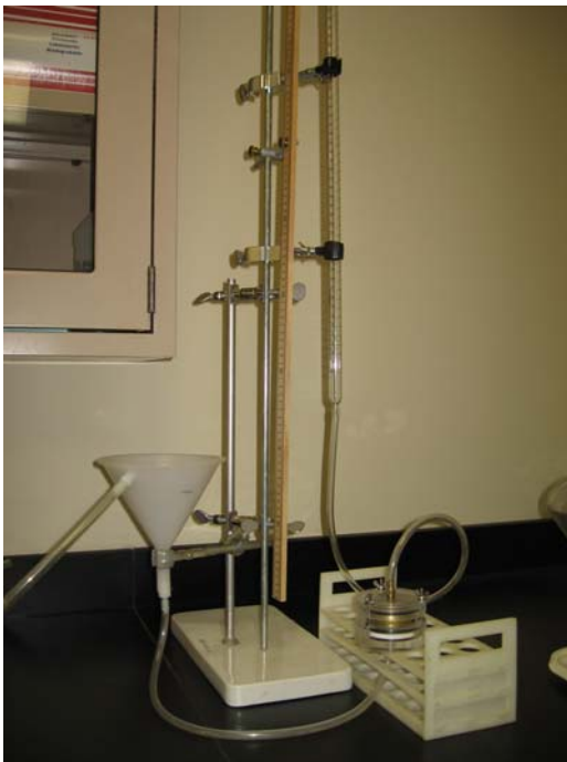
Figure 8: Equipment set up for determining the permeability for the native soil using the falling head permeameter
