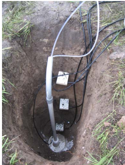
Figure 7: Tensiometer at the 3-ft depth with TDRs (porous element)
