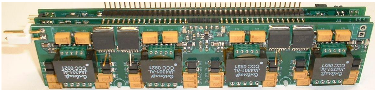
Figure 144 Picture of the boards with components (left: top side, right: bottom side, top: control board, middle: driver board, bottom: isolated power supply board)
