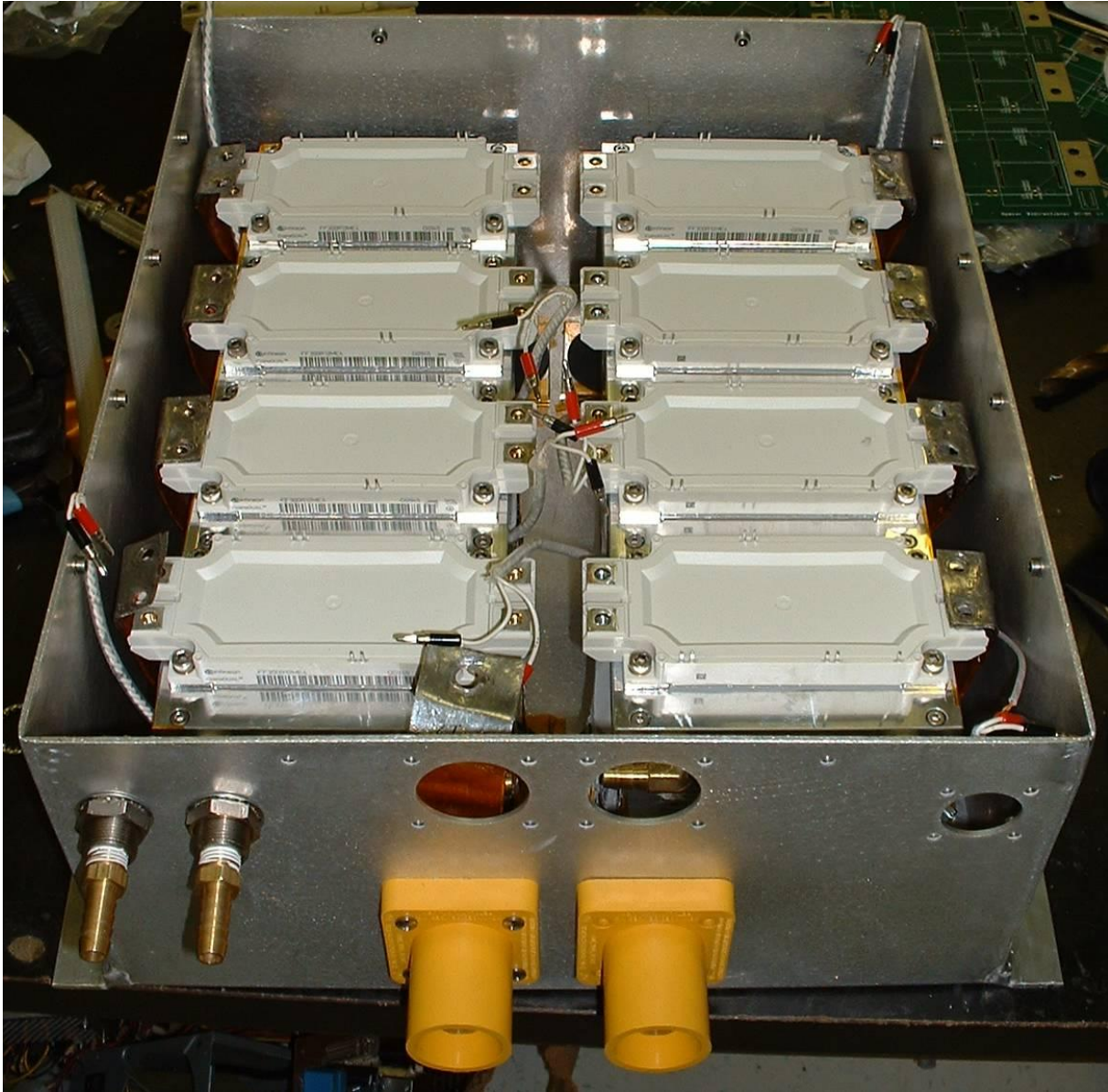
Figure 151 IGBT modules mounted to coldplate assemblies
