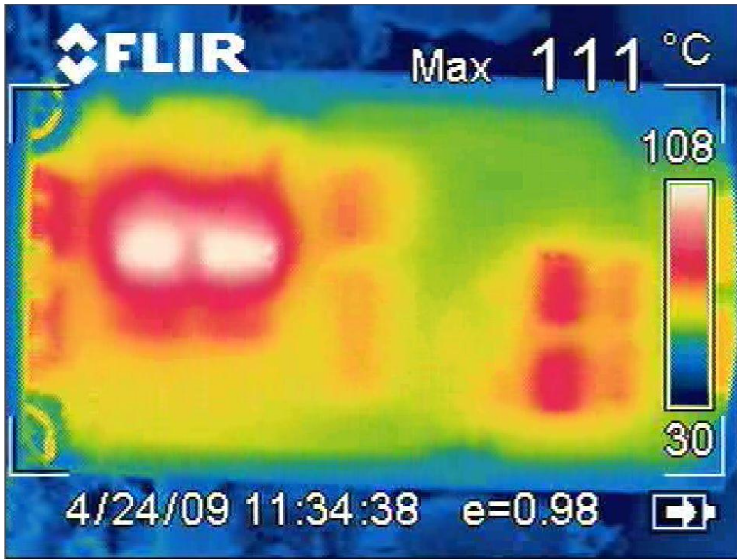
Figure 120 Thermal image of Powerex CM300DX-24A IGBT @ 21kW and 70°C cooling
