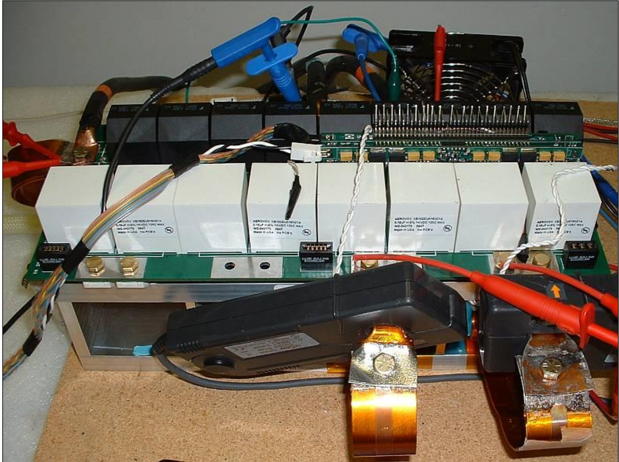
Figure 136 Initial power PCB testing setup
