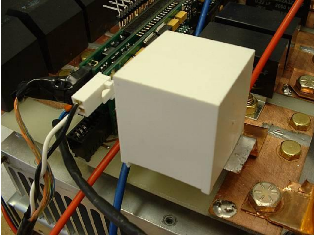
Figure 128 Test setup to evaluate new snubber capacitor
