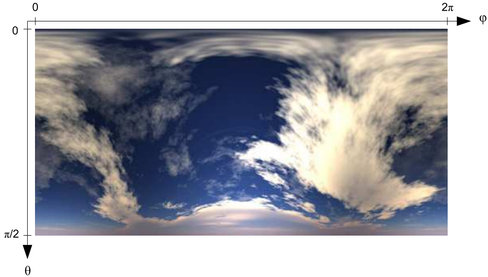
Figure 2.7: Example of latitude-longitude mapping for environment lighting using a hemisphere. The lower part of the environment sphere is set to 0 in this case.
