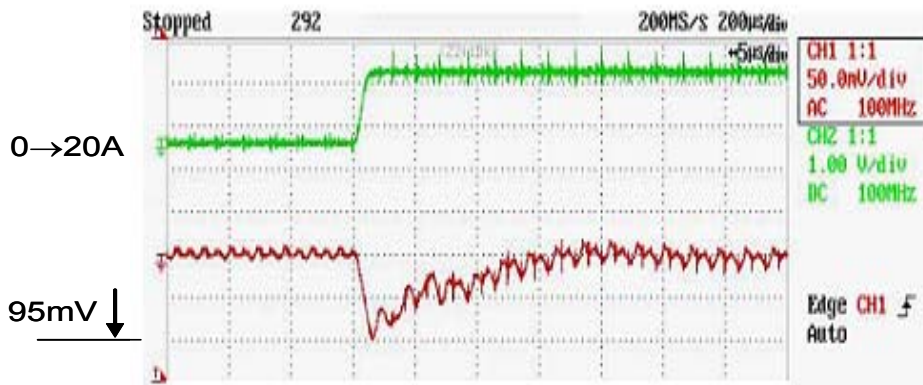
Fig.4.2.10 Output ripple in step-up load @10A/ \mu s
