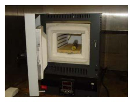
Figure 3.14: Mandrel containing coiled SMA wire in the furnace
