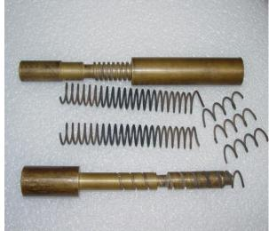
Figure 3.13: Helical shape memory alloy actuators and spring winding mandrels
