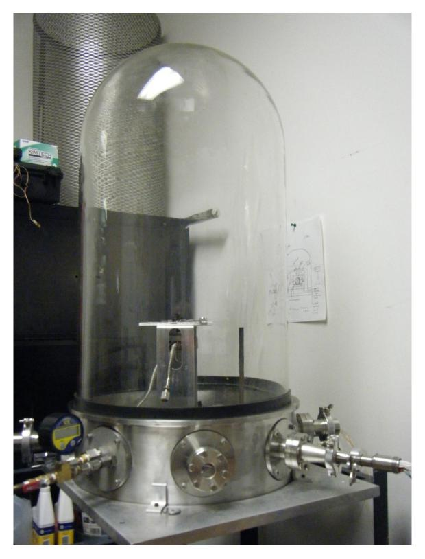
Figure 6.6: Glass bell jar with instrumentation feedthroughs
