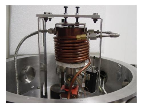
Figure 6.8: Thermal switch and single-loop cooling coils connected to liquid nitrogen lines
