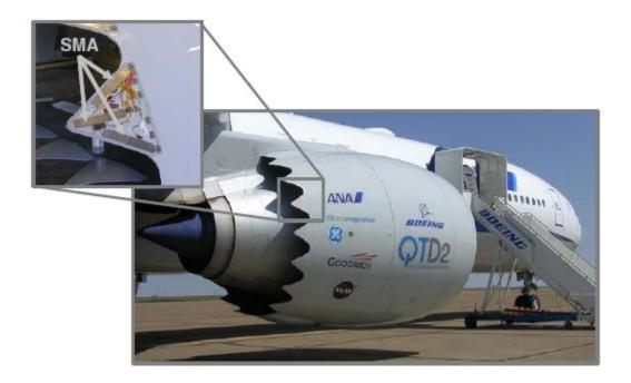
Figure 2.5: Shape memory alloy actuated variable geometry chevrons [26]
