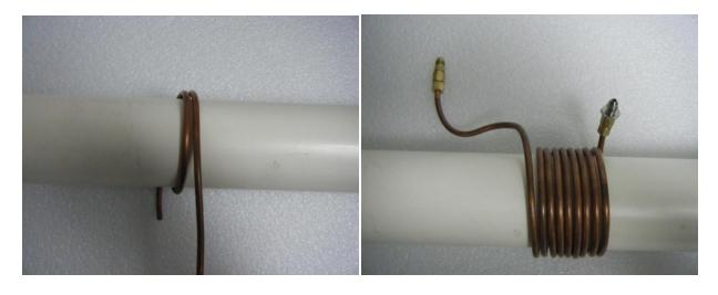
Figure 6.5: Fabrication of the single-loop copper tube
