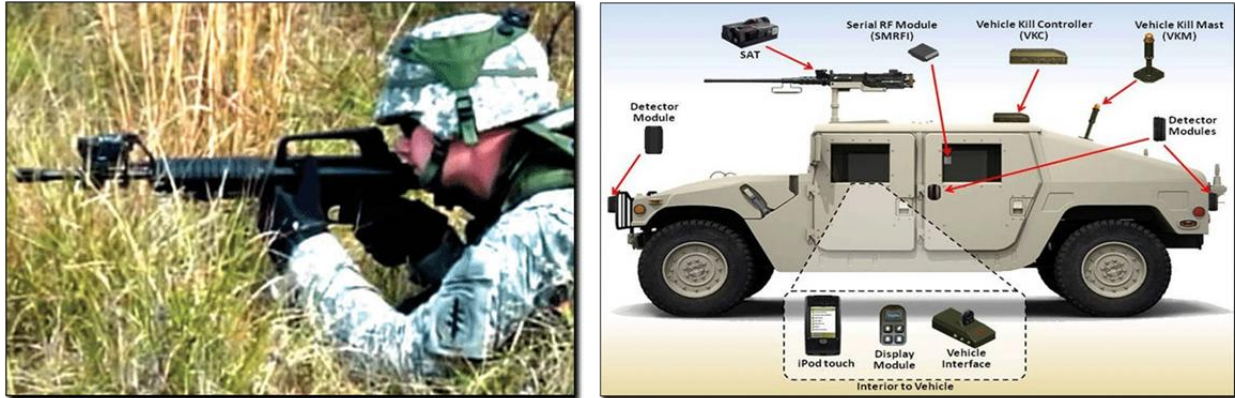
Figure 1: IMILES-IWS mounted on 25th ID Soldier's weapon and Kevlar; IMILES-TVS fitted on a HMMWV (LTS, Live Training Systems).
