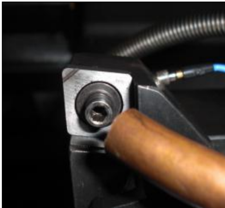
Figure 15: Groove Location for Thermocouple on Insert
