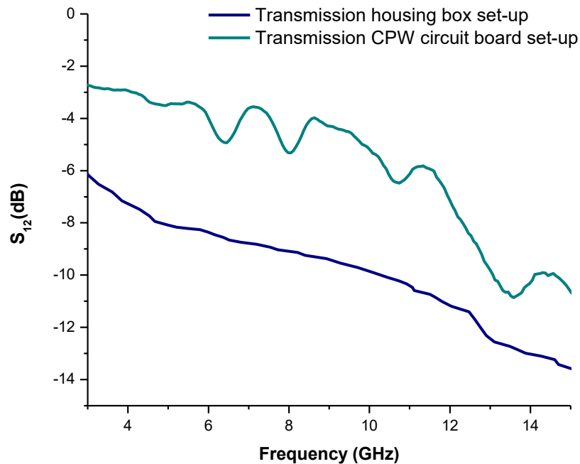
Figure 23: Comparison between the transmission of the sample when wire bonded into the circuit board and the transmission of the sample when placed in the housing box.
