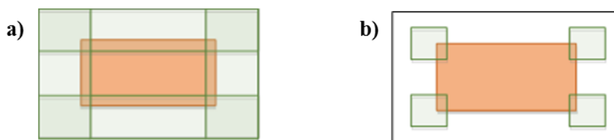
Figure 64: Illustration showing the graphene/Cu foil tied on plastic with Kapton tape ready for spin coating. b) Graphical representation of how to prepare the graphene/Cu for etching.
