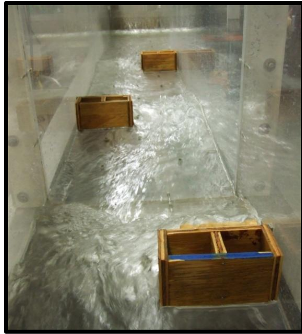
Figure 40: Flume Testing for Staggered Configuration
