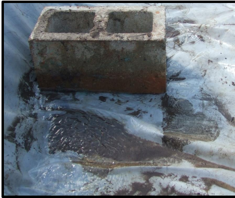
Figure 59: Floc Accumulation using A-3 Soil
