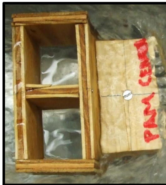
Figure 11: Image of Wood Replication of Obstruction for Flume
