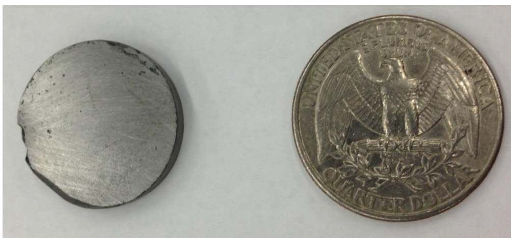
Figure 58: The \text{OsB}_2 sample after spark plasma sintering (left), and a US quarter coin (right) for comparison of the sizes.
