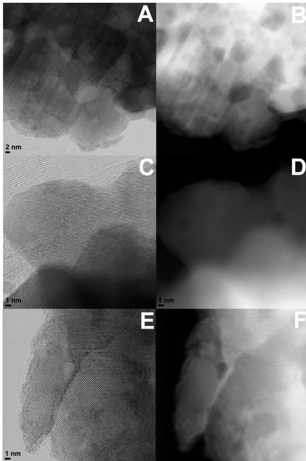
Figure 90: Bright field (A, C and E) and dark field (B, D and F) STEM images of hexagonal OsB 2 .
