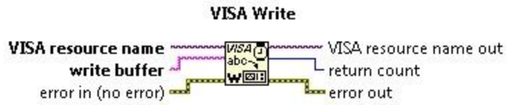
Figure B. 3: VISA Write Writes Data to the Specified Port by the VISA Resource Name
