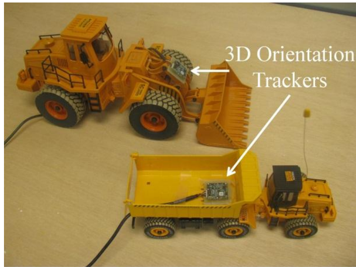
Figure 6.6: Orientation Trackers Mounted on a Loader's Boom and a Truck's Bed
