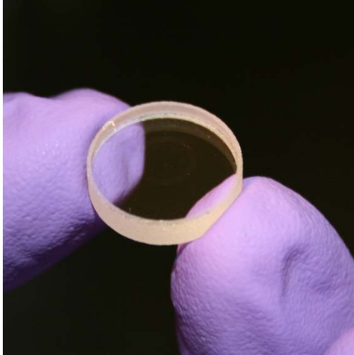
Figure 7.2. Photograph of the DOE zones fabricated on a half-inch fused silica substrate.
