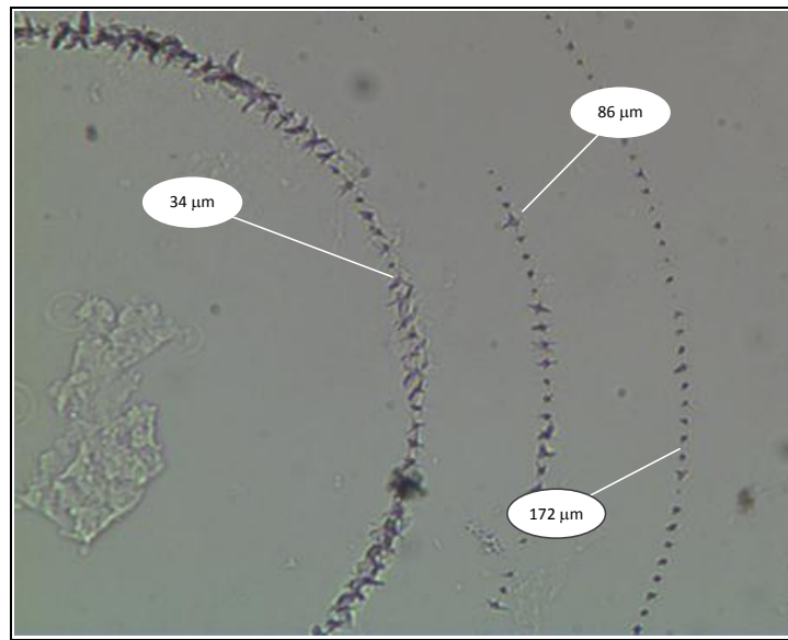
Figure 115 Capsulotomy pattern in porcine capsule at laser fluence of 25.3 \text{ J/cm}^2 at axial, z, spacing indicated.
