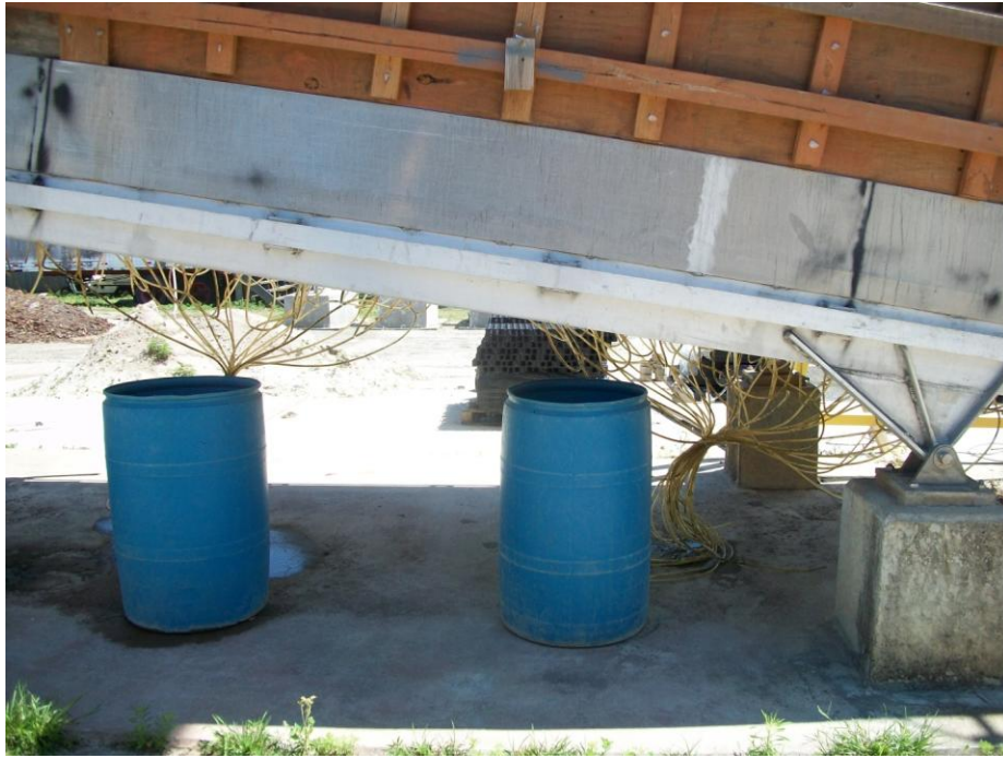
Figure 16: Baseflow Collection Tubes and Barrels
