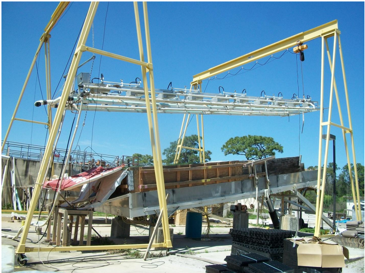
Figure 7: Side View of Test Bed, Rainfall Simulator, and Gantry Crane
