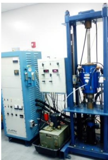
Figure 10 Hot-press (Thermal Technologies, Inc.) used for initial sintering experiments.
