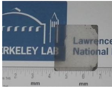
Figure 7 2x2 mm melt-quenched lanthanum stabilized, europium doped BaCl 2 ceramic synthesized at LBNL. The picture was provided by LBNL colleagues Drs. E. Bourret and Gregory Bizarri.
