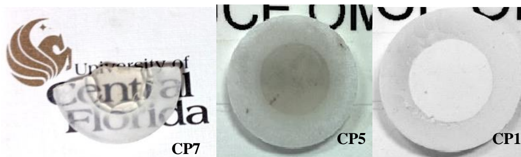
Figure 33 A comparison of 2 mm-thick samples sintered using coarse \text{NaCl} and \text{BaCl}_2 powders (CP7), fine \text{BaCl}_2 powders (CP5), and fine \text{NaCl} powders (CP1).
