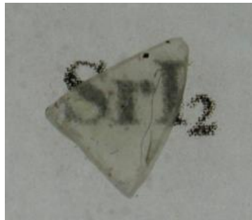
Figure 8 Transparent \text{SrI}_2 ceramic produced by hot-pressing [37]. Picture provided courtesy for Prof. Romain Gaume
