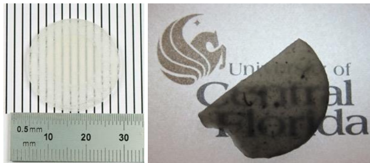
Figure 52 Sample EU3 prepared from a crushed high-quality single crystal (left) and sample EU4 prepared in the commercial hot-press (right).
