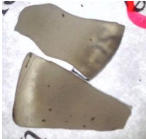
Figure 15 Sample prepared by cold-pressing, conventional sintering at 750°C, followed by a hot-forging operation at 750°C.
