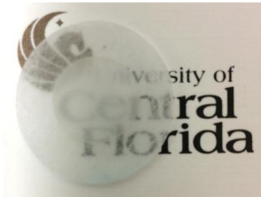
Figure 31 Ceramic sintered from spray dried powder at 450°C and 120MPa (SD1).
