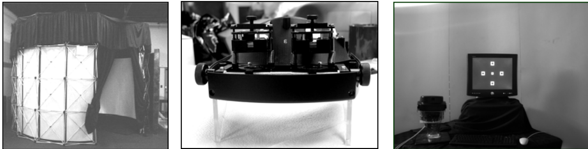
Figure 38 VE system: ARC, HMPD, and computer setup
