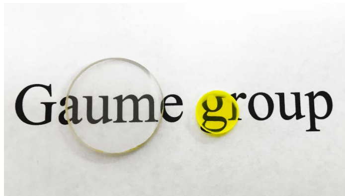
Figure 1. Transparent YAG fabricated in our lab. Right Ce:YAG and left Tm:YAG
