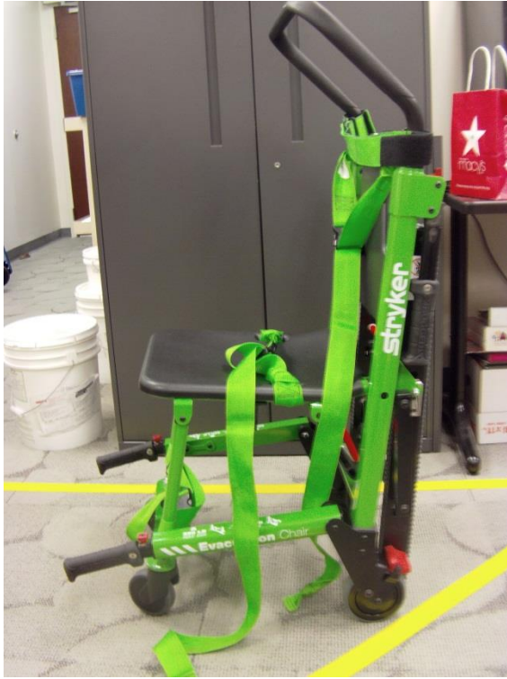
Figure 1: Stryker Step 1—Pull Seat Down
