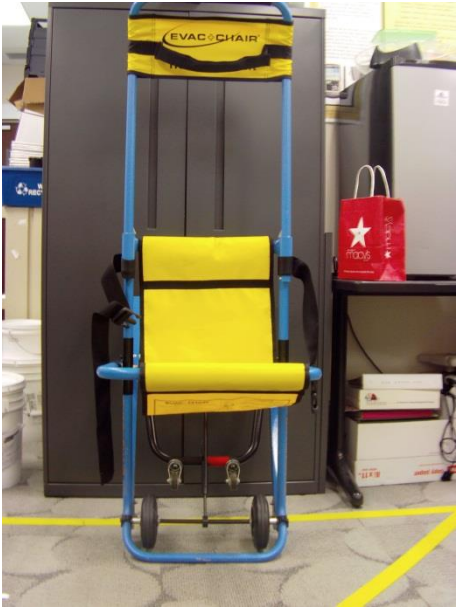
Figure 11: Evac+chair Step 5—Pivot Seat Frame Down
