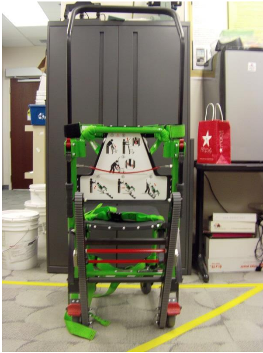
Figure 3: Stryker Step 3—Grip Horizontal Red Bar, Squeeze to Release Track
