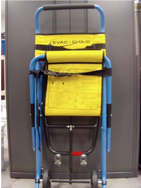
Figure 7: Evac+chair Step 1—Place Foot on Bottom Bar
