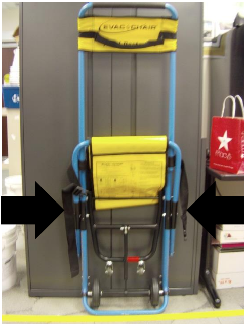
Figure 10: Evac+chair Step 4—Unbuckle Seat Belt
