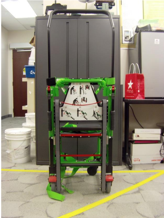
Figure 2: Stryker Step 2—Extend Top Bar by Pulling Red Wire Upward While Pulling Top Bar Up
