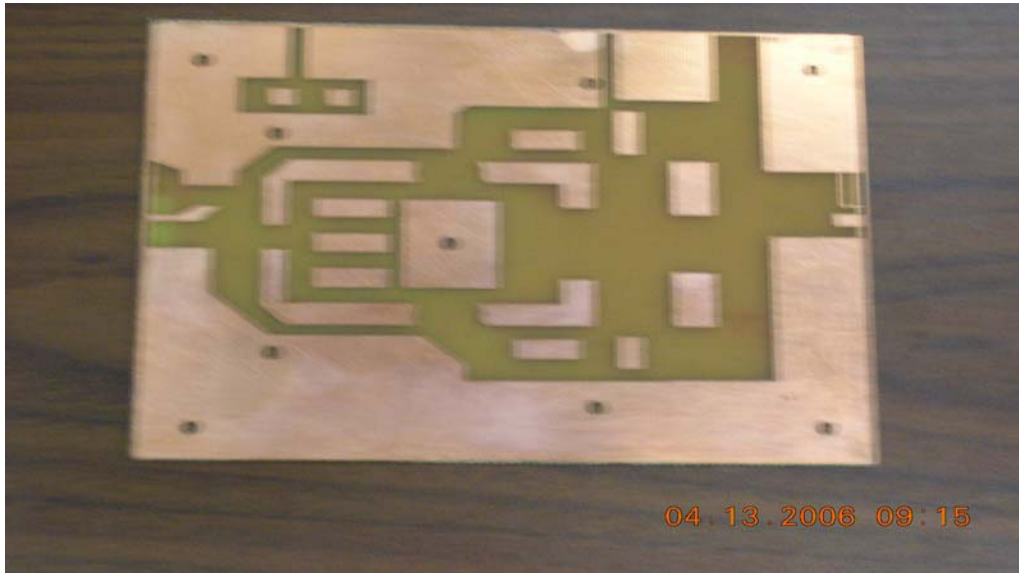
Figure 50: Etched layout of the coupling unit
