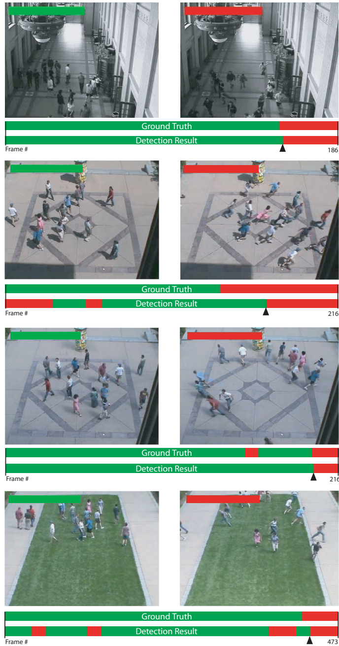
Figure 3.7: The qualitative results of the abnormal behavior detection for four sample videos of UMN dataset. Each row represents the results for a video in the dataset. The ground truth bar and the detection bar represent the labels of each frame for that video. Green color represents the normal frames and red corresponds to abnormal frames. The left column shows the first frame of the video and the right column is the first frame of the detected abnormal block (black triangles).
