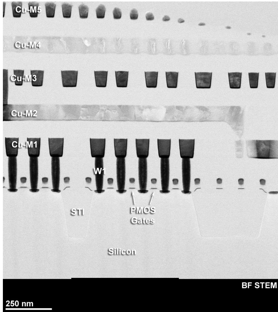
Figure 10-15 Bright field STEM image of PMOS gates and upper metal and dielectric layers.
