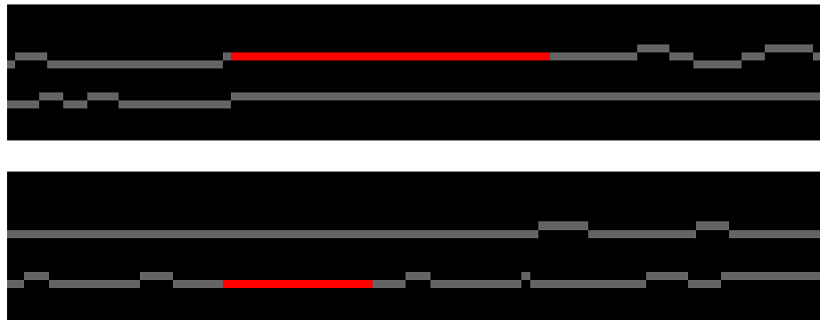
Fig. 3 Examples of Connecting Two Edges With Same Parallel Partner
