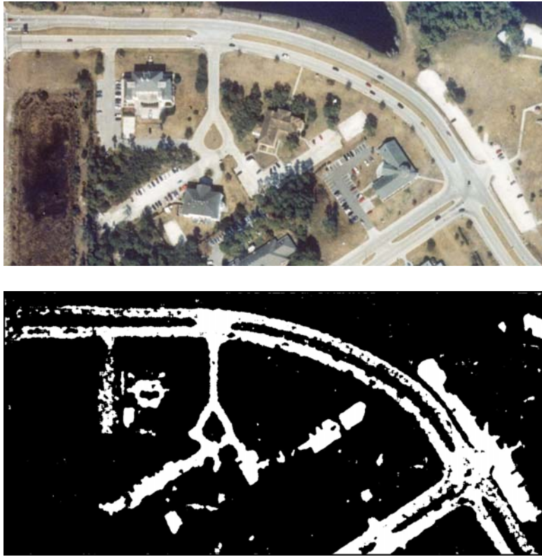
Fig. 13 Example of Failing Texture-Based Segmentation (2)
