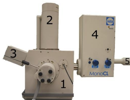
Figure 6. This is the Phillips XL30 SEM workstation used during the experiment. This station includes the SEM vacuum and sample chamber (1), electron beam column (2), secondary electron detector (3), Gatan Mono CL3 monochromator (4) and the Hamamatsu photomultiplier tube (5).
