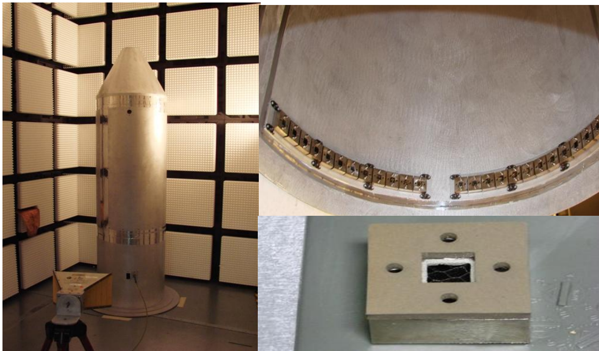
Figure 86. Test set-up and fixture showing the honeycomb inserts for RF hardening.
