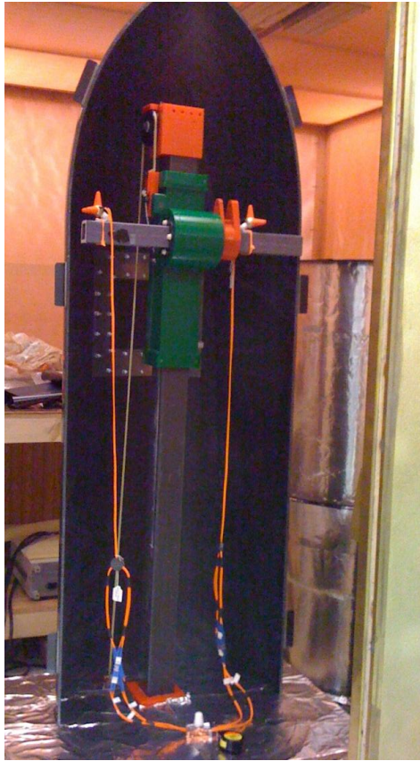
Figure 45. Composite fairing half test set-up with fiberglass mount and outer probe positions.
