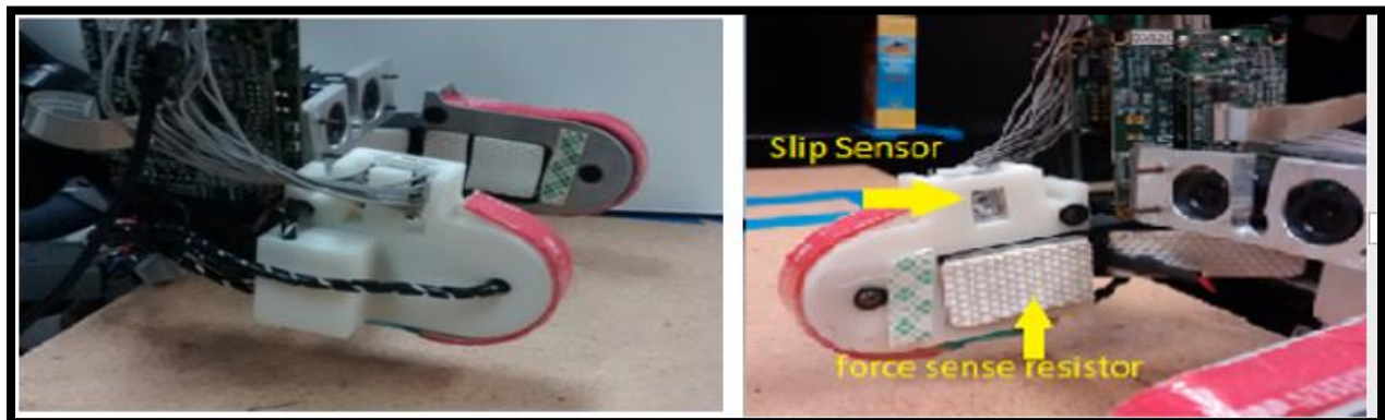
Figure 8: Proposed Model-1 for Laser Sensor-FSR Sensors (Phase-1 Experimentation)
