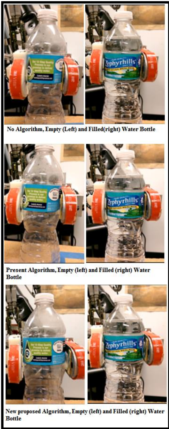
Figure 16: Pictures showing Grasping Operations on Water Bottle
