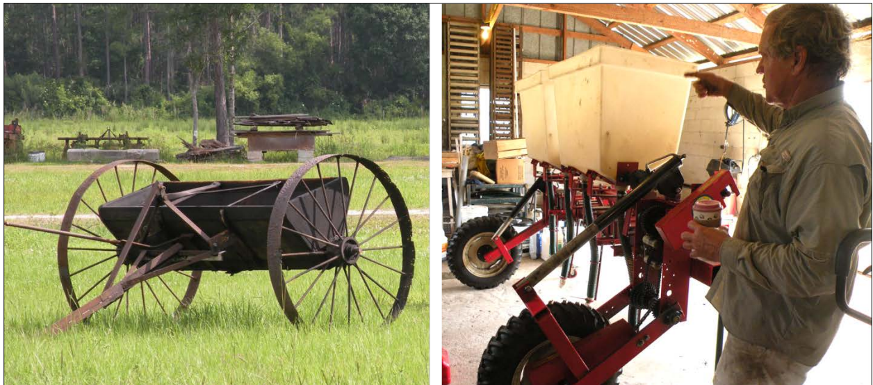
Fig. 8. Comparison of Seed Drills on Tomazin Farm. Left: early model, modified for raised-bed farming. Right: Bill Tomazin describes the operation of his new hydraulic drill seeder.
