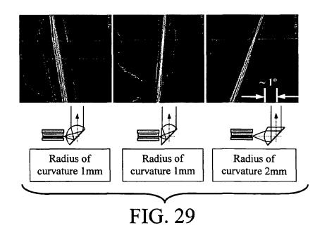
Experimental result of different beam control prism designs
