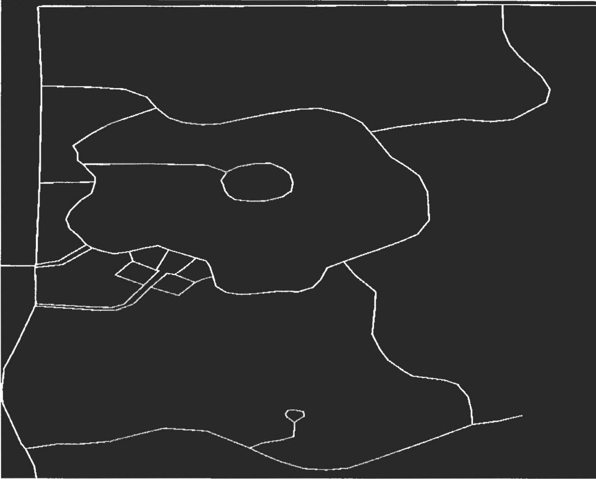
Fig.9 The database for the area of UCF campus. All the roads were obtained from aerial image by using our own software. Note that only some roads in the area are included and the present terrain is at the very low level of detail (two triangles).
