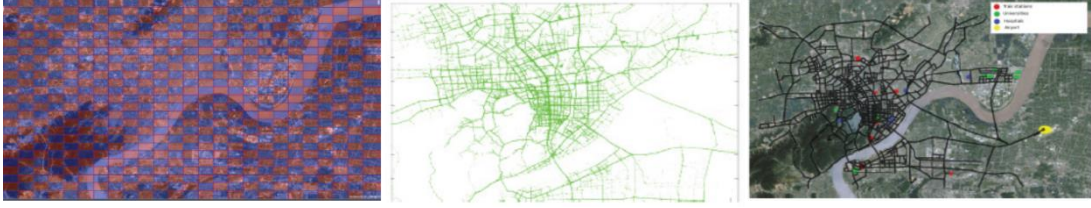
Figure 1: Grid decomposition (left), traces from 20 taxis (center) and digitized road network (right) for the city of Hangzhou, China.
