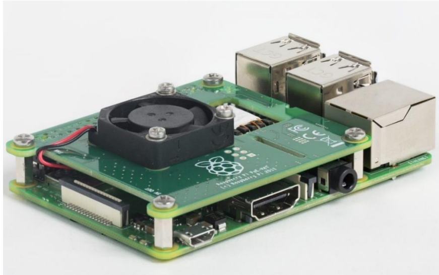
Figure 7 – HAT attached on the RPi 3 Model B+ [91]
