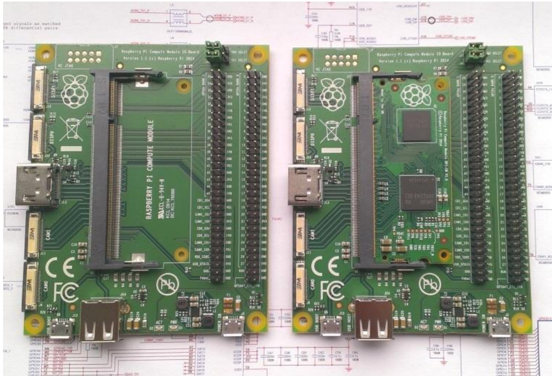
Figure 8 – IO Module board (Unpopulated & populated) /w the Compute Module [100]
