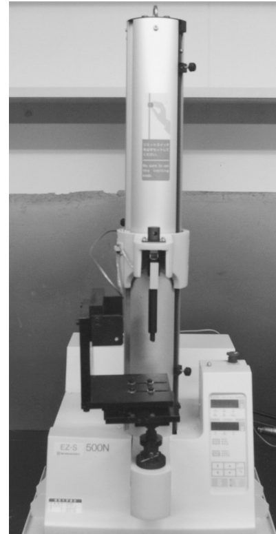
Figure 4 The electronic universal testing machine (EZ-Test ; Shimadzu, Kyoto, Japan)
