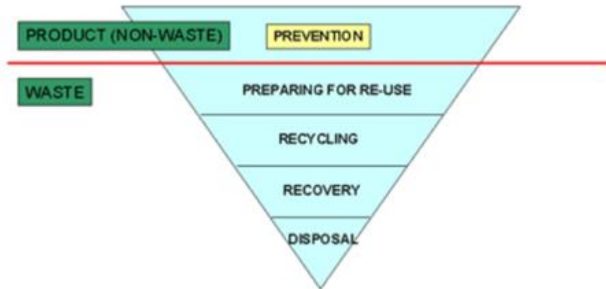
Figure 4: The waste management hierarchy according to EU, source: EU Waste Framework Directive
