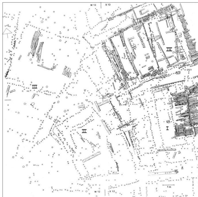
Fig. 39 Plan of the architectural remains (postholes, wooden floors and foundations) in phase VIII (Thissen 2001, 304).
