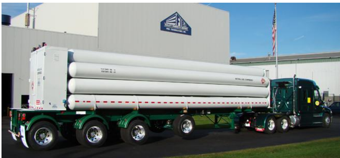
Picture 4: CNG trailer.
