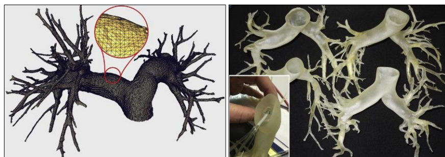
Figure 9: Preplanning in thoracic surgery, Rendered triangular surface and 3D-model of the pulmonary artery, Source: (Kurenov et al. , 2015)
