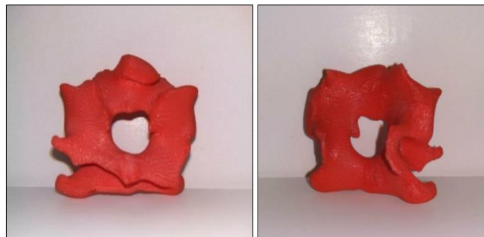
Figure 198: The final 3D-printed model of the T4 vertebra, Anterior and Posterior Side
