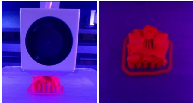
Figure 197: The 3D-printing process of the T4 vertebra via BCN3D Sigma R17 printer
