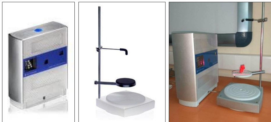
Figure 199: Next Engine 3D Scanner Source: [28], Placement of the T4 vertebra in the Auto-positioner of the scanner
