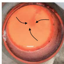
Fig. 7: Photograph of inductively stirred NaCl-KCl melt.
