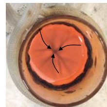
Fig. 8: Photograph of inductively stirred vanadium oxide melt.
