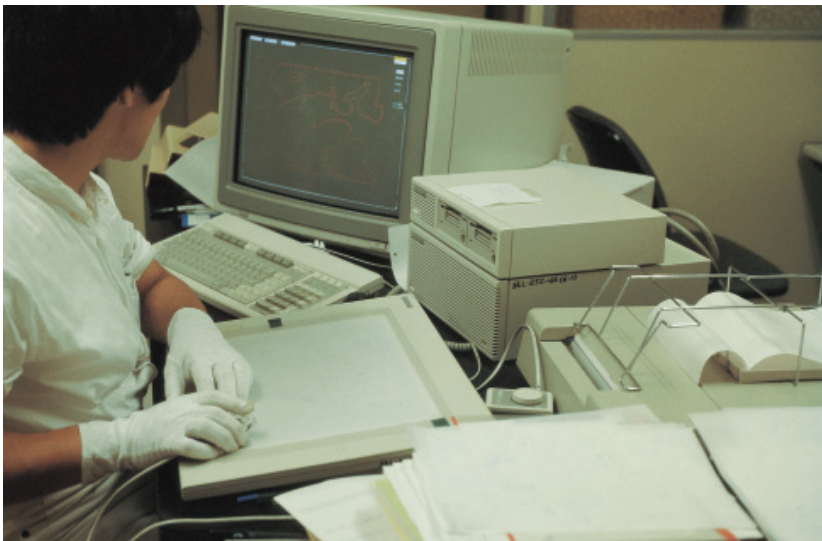
Fig. 4-8. A system designed to assist the analysis of 3-D organ structure (OZ system, produced by Rise).
