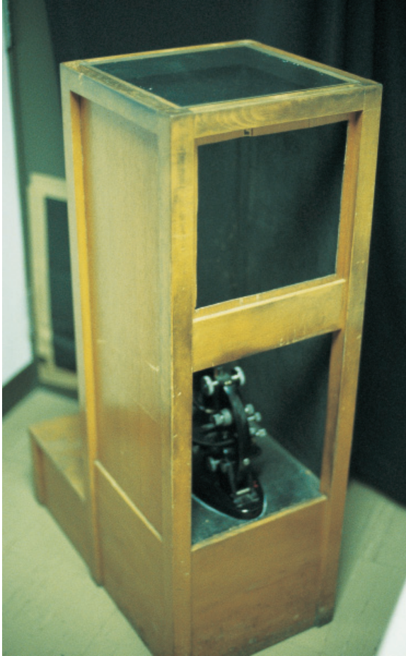
Fig. 4-4. A makeshift projector making use of a monocular microscope, equipped with Köhler illumination.
