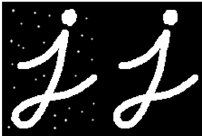
Fig. 1.12 Application of mathematical morphology to filter small blobs in a binary
