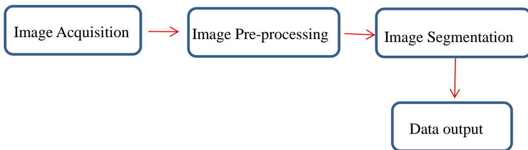
Fig. 1.7 Typical procedures in image processing method.
