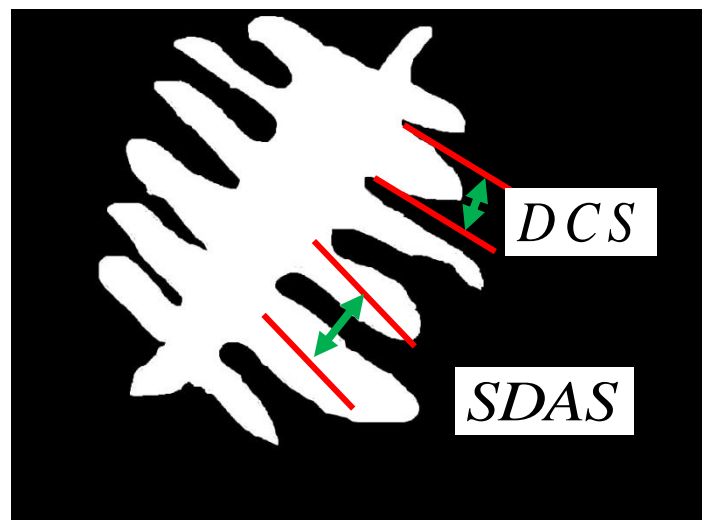
Fig. 4.1 Schematic for SDAS and DCS in a dendritic structure.
