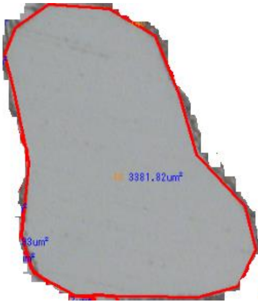
Fig. 2.6 Manual measurement result of primary grain size distribution.
