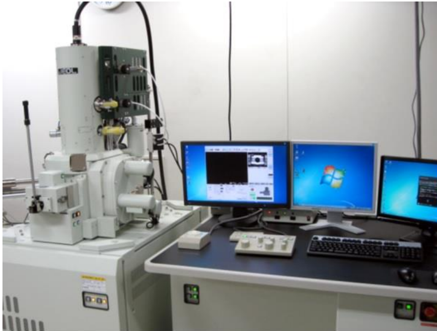
Fig. 2-10 Overview image of SEM, JSM-7100F (2-3) .
