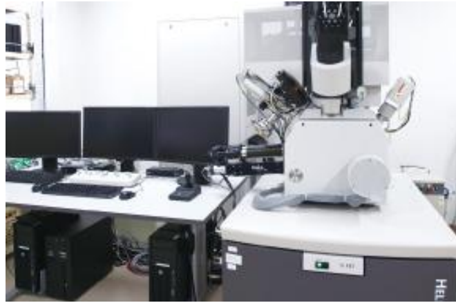
Fig. 2-12 Overview image of FIB apparatus, Helios NanoLab™ 600i (2-5) .
