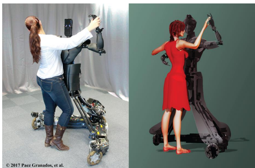
Figure 1: Robot Dance Teacher (roboDANTE). Left side: photograph with a human partner. Right side: robot CAD accompanied
