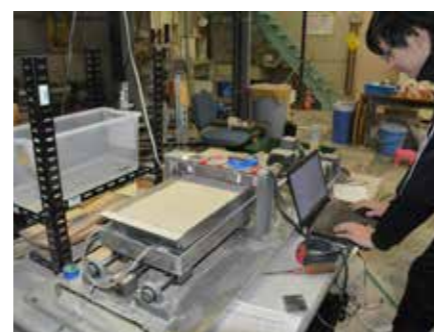
Fig.3 Excavation experiment of the soil in water
