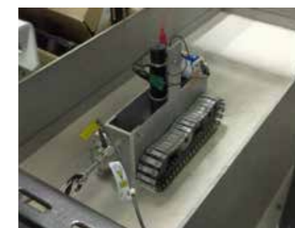
Fig.5 Tractive force measurement experiment
