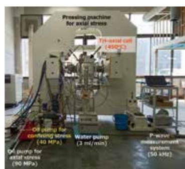
Fig.3 Large-scale hydraulic fracturing experiment under supercritical condition.
