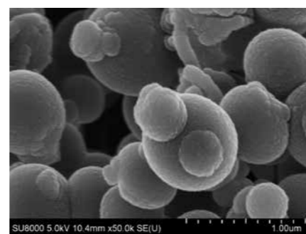
Fig.3 SEM photo of silica particles produced by flashing experiment from supercritical fluids.
