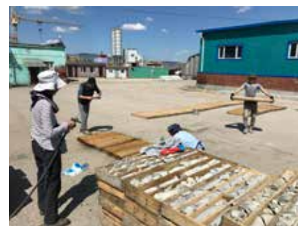
Fig.1 Sampling from the porphyry copper deposit cores of Erdenet mine, Mongolia.
