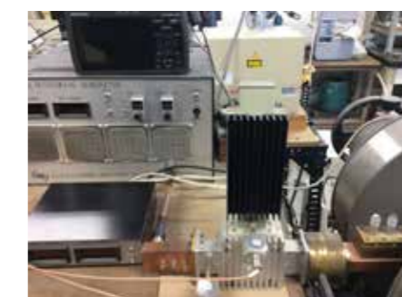
Fig.4 Microwave processing apparatus with imposition of static magnetic field
