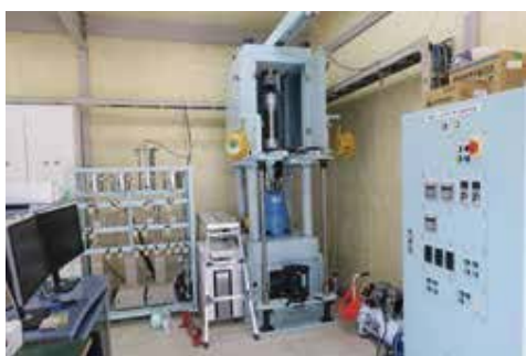
Test facility of mechanical/hydrological behavior of rock
