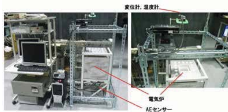
Fig.2 Evaluation system for deformation/temperature/AE of SOFC planer cell.
