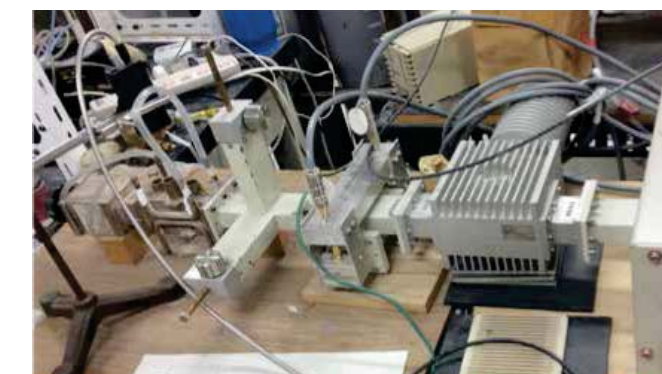
Fig.5 Microwave single mode applicator of 5.8GHz for rapid synthesis of ZrB 2 ceramics.
