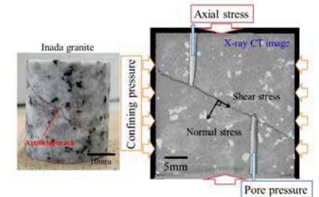
Fig.5 Granite specimen for slip experiment.
