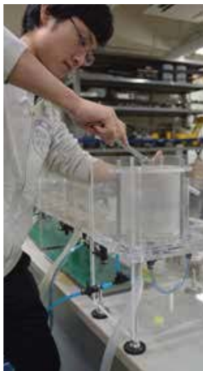
Fig.1 New developed permeability test apparatus
