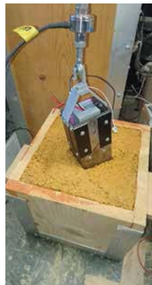
Fig.4 Soil sampling test using developed device
