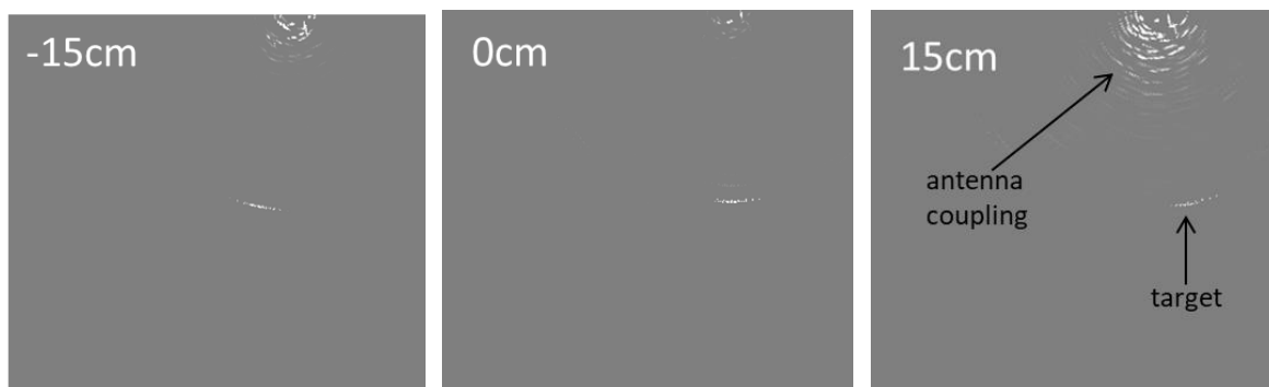
Figure 62 Reconstructed image using caustic finding algorithm.
