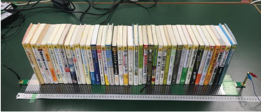
Figure 2.26: Experiment environment of smart-shelf system using switching reception.
