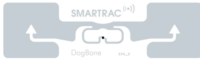
Figure 3.4: Geometry of an commercial RIFD tag.
