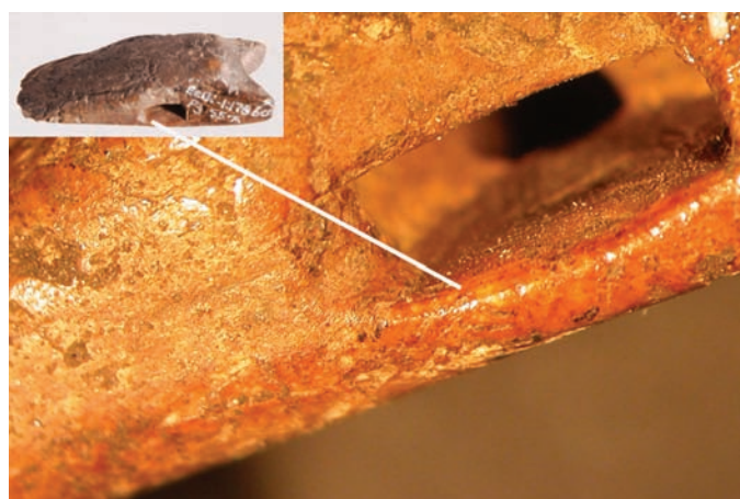
FIG. 4. Magnified (10×) view of a line hole on a line fastener showing polished edge.
