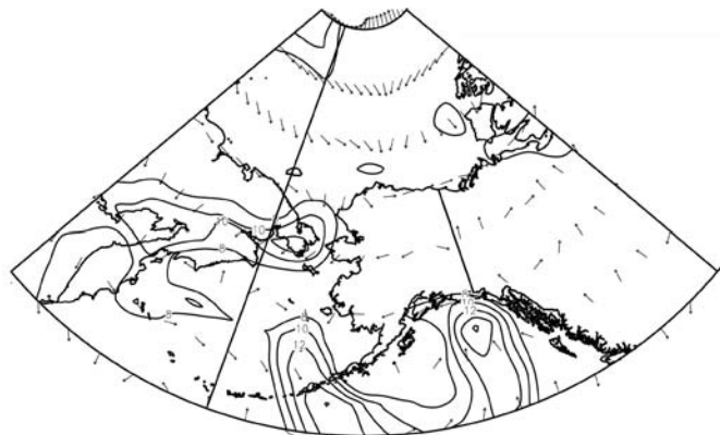
FIG. 3. Surface winds (10 m height) associated with the in situ slush-ice berm event of 10 November 2012 at Wales, Alaska. Small arrows indicate the direction of the wind. Contour lines indicate wind speed in meters per second (m/s). Only wind speeds of 8 m/s or greater are displayed. Contour interval is 2 m/s. Data from NOAA/ESRL.
