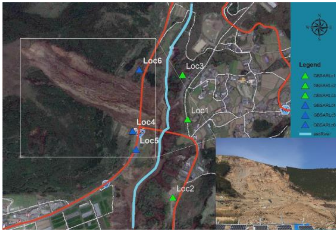
Figure 3.10 The proposed location for GB-SAR installation was shown in Loc1 to Loc6 which located in left side (blue) and right side (green) to the Kurokawa River .
