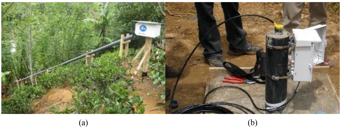
Figure 7.5 existing landslid monitoring method (a) extensometer (b) stringauge
