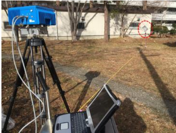
Figure 2.7 Experimental setup of GB-SAR calibration
