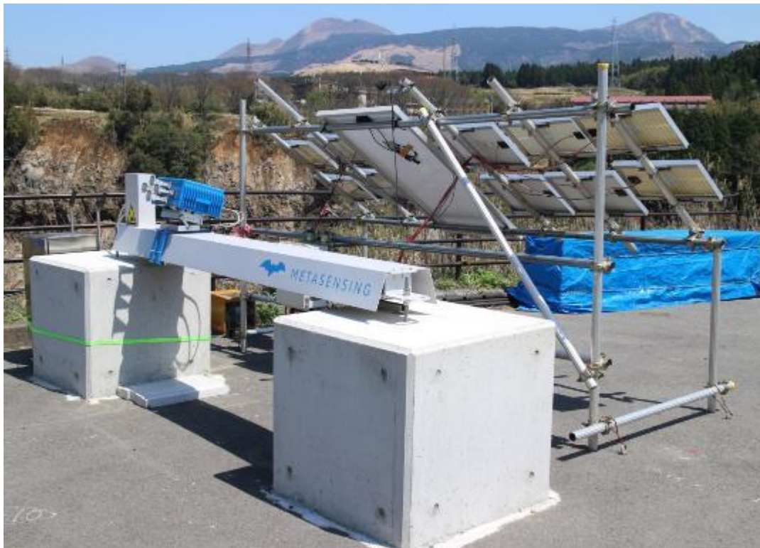
Figure 6.1 GB-SAR system deploy in Minami-Aso
