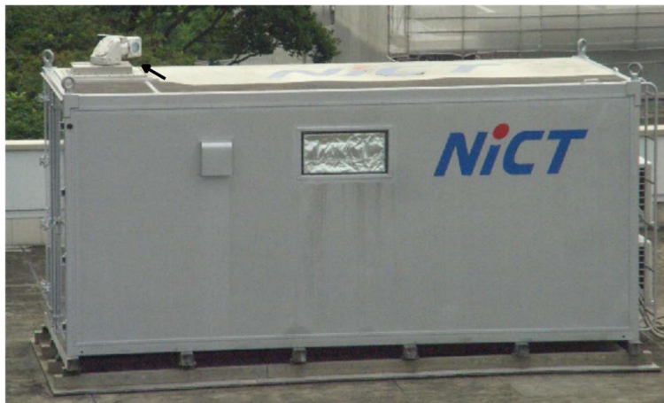
Figure 2.3. Photograph of Co2DiaWiL stationed on the rooftop of a building at NICT headquarters from 2010 to 2012. The container houses the transmitter and receiver, and the scanner is installed on its roof. The arrow points to the scanner.
