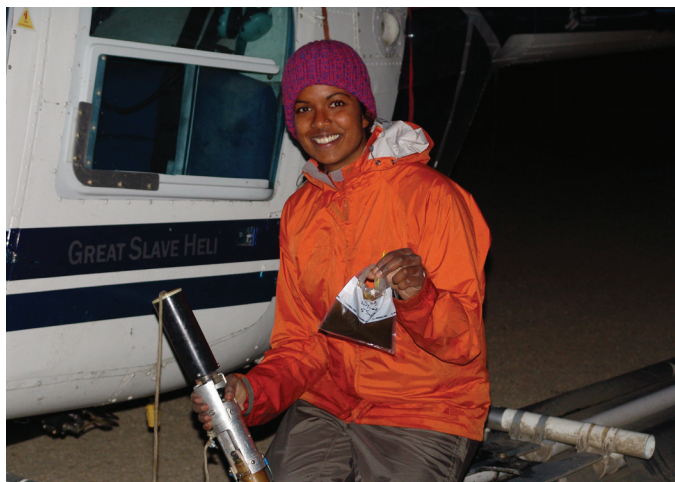
FIG. 3. Ann holding a sample of surface sediments taken using a gravity corer. Photo by Roland Hall.
